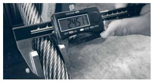
Figure 12: Small caliper with wide measuring surfaces
