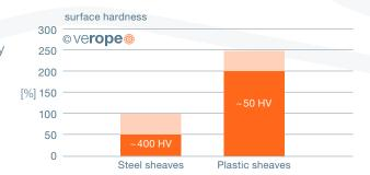
**Figure 49:** Influence of the sheave material onto the rope lifetime
