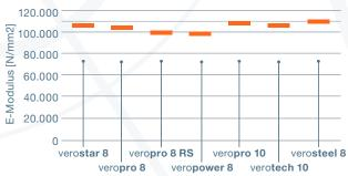
**Figure 55:** E-Modulus rotation resistant ropes
