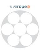
Usually fill factors of wire ropes with a wire rope core increase with an increasing number of outer strands. A rope of the design 6x25 Filler-IWRC has a fill factor of 0,58 and a rope of the design 8x25 Filler-IWRC has a fill factor of 0,587.
