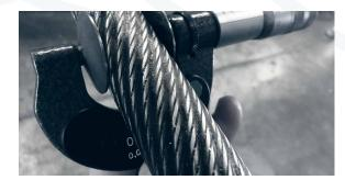
Figure 11: Micrometer with wide measuring surfaces
