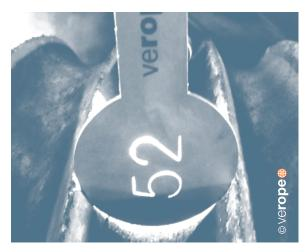
**Figure 74**: Groove gauge (shown in a too narrow groove)
