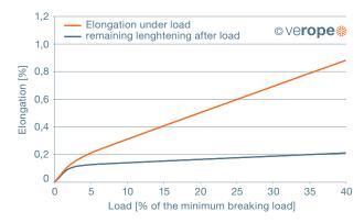
**Figure 57:** Elongation under load (upper graph) and remaining lenghtening after load (lower graph) depending on the line pull (vero**top P** , lang's lay, 1960 N/mm2)
